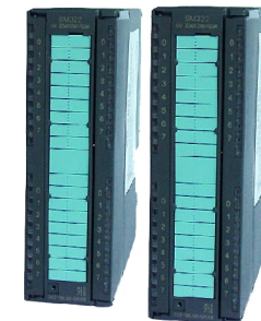
CTS7322-1BL00 EM322, 32DO × 24VDC, Optical Isolation, 40PIN front connector
